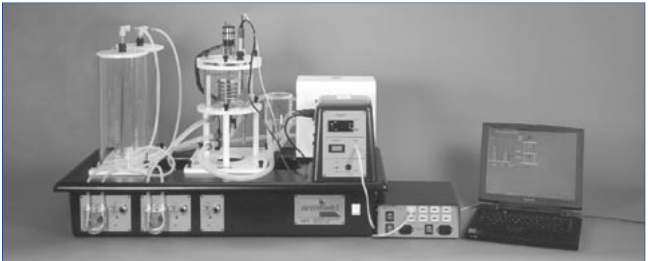
CEX service unit shown with the CEM MkII reactor installed and connected to a computer through an IFD6 interface device.
