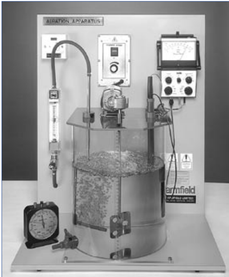
The Aeration Unit with sparger tube diffuser installed
